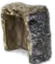
CHEC-1 CHARRED VALVE COVER
